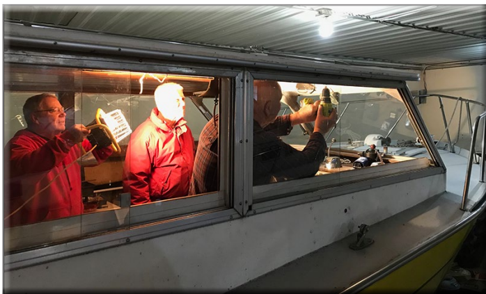
PC Mike Muhn holds the light as Paul Kalister and John Eschels install headliner slats on Escort III .
